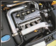
Above: when 210bhp isn't enough - enlist forged pistons and Carrillo rods together with hybrid turbo at 2.2bar for 400bhp
